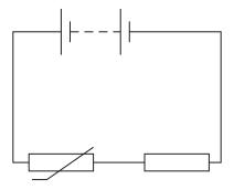
At a temperature of  $45\,^{\circ}$ C, the resistance of the thermistor was four times the resistance of the resistor. The power *P* dissipated in the resistor was  $0.38\,\text{W}$ .
