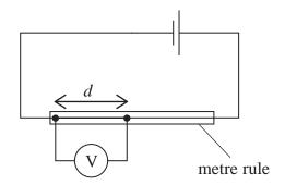
The distance d between the connections to the voltmeter is increased. The reading V on the voltmeter changes.
