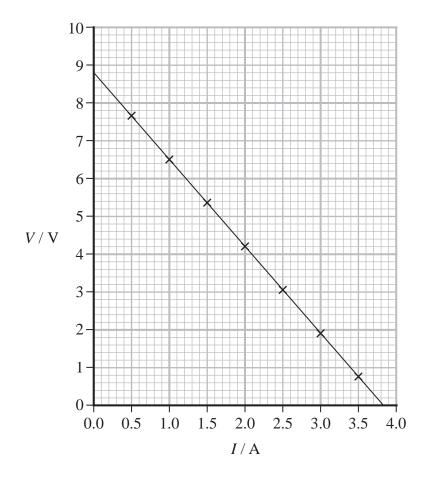
(i) Determine the e.m.f. and internal resistance of the battery.
