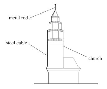
When lightning strikes, charge is transferred to the metal rod and is conducted to the ground through the steel cable.
