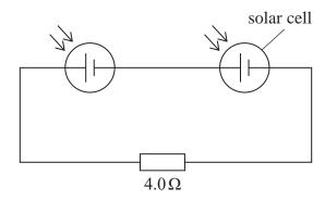
The student adjusted the light conditions so that each solar cell had an e.m.f. of  $5.0\,\mathrm{V}$  and an internal resistance of  $0.80\,\Omega$ .
